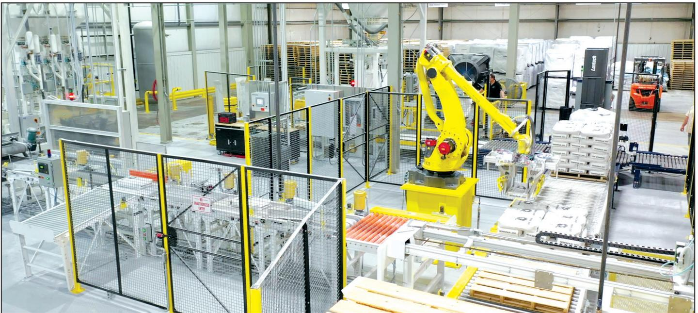
Magnum Systems' total system solution for moving and bagging mineral products in 50 lb and 1,000 - 2,000 lb bulk bags from start to finish at The Quartz Corporation.
