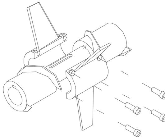
Figure 7-15. Impeller, Exploded View
