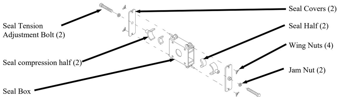
Figure 7-22. Impeller Shaft Seal, Exploded View
