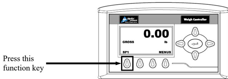
Figure 4-7. Initial Setup – Single Set Point
