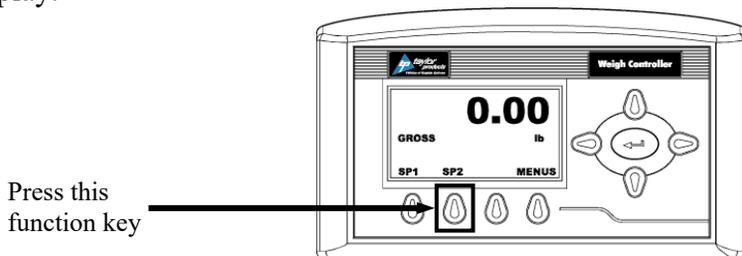
Figure 4-12. Setting the Target Weight (SP2)
