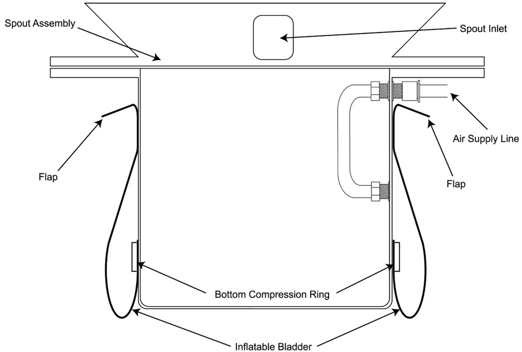
**Figure 7-9.** Pulling the Bladder Up, and Creating the Upper Flap
