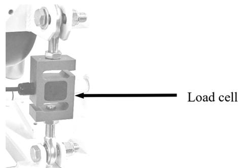
Figure 1-4. Load Cell
