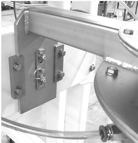
Figure 7-5. Open Mouth Bag Spout Mounting Bracket
