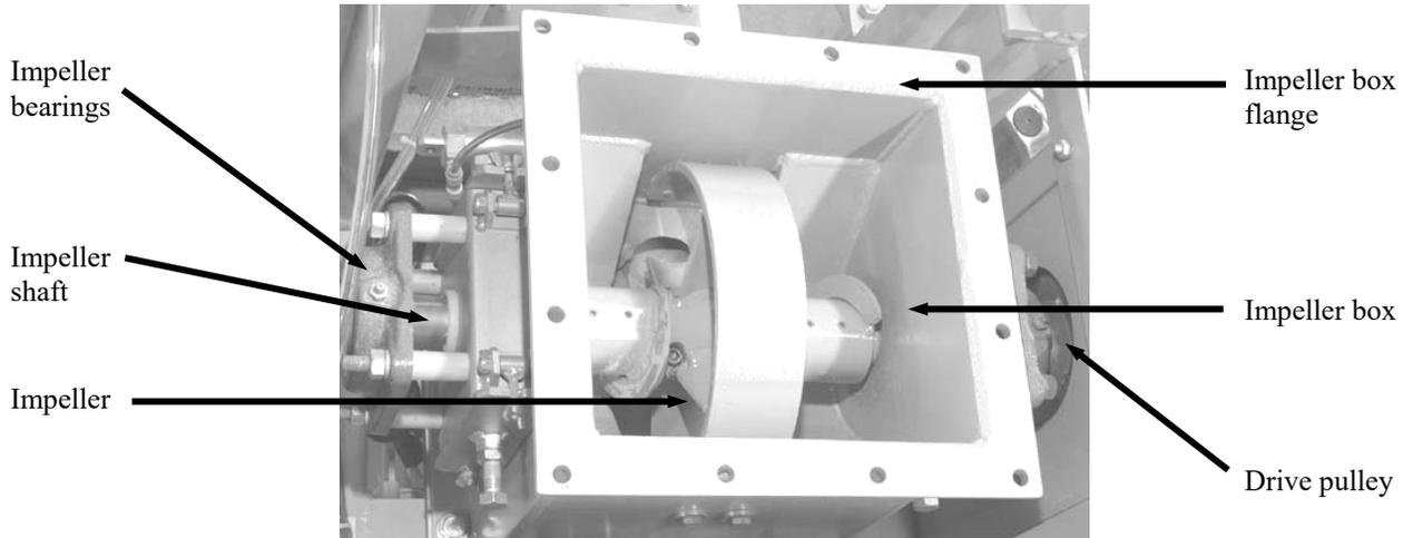
**Figure 1-3.** Impeller Assembly
