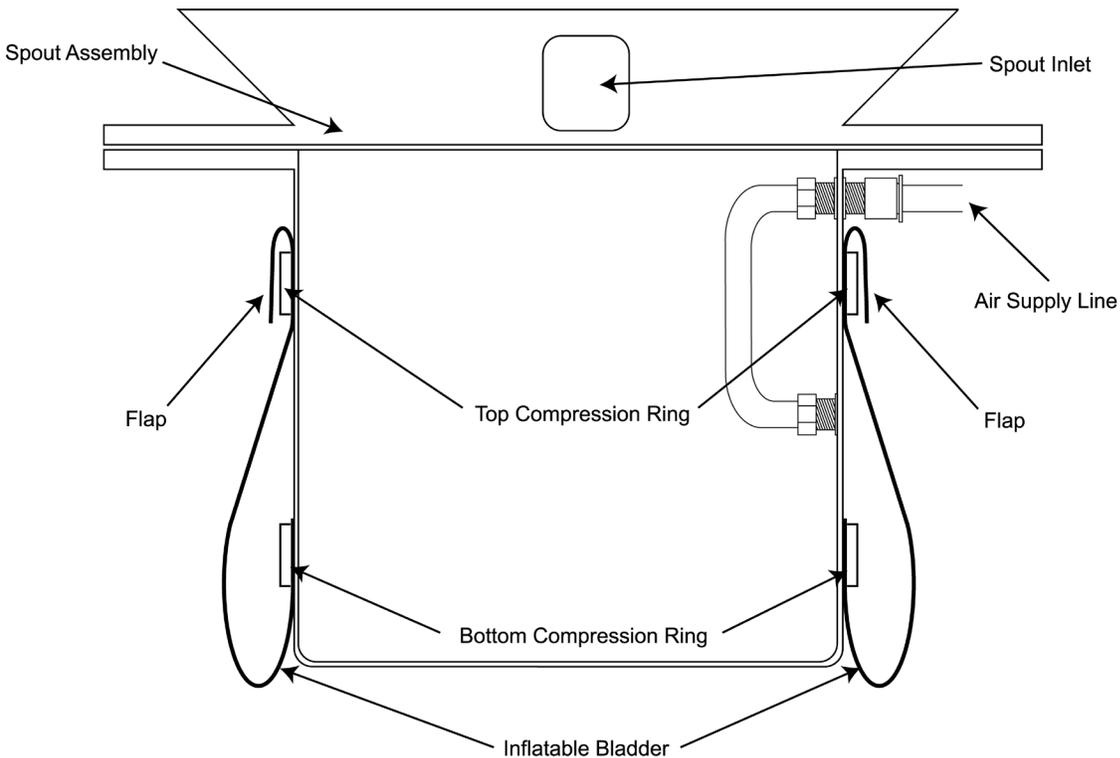
**Figure 7-6.** Section View of Open Mouth Bag Spout and Inflatable Bladder
