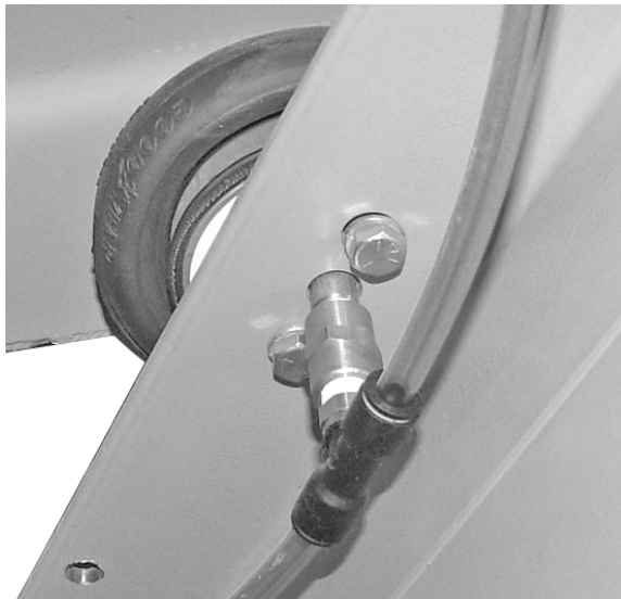
Figure 7-11. Lower Air Mount Isolator Mounting Bolts and Air Fittings
