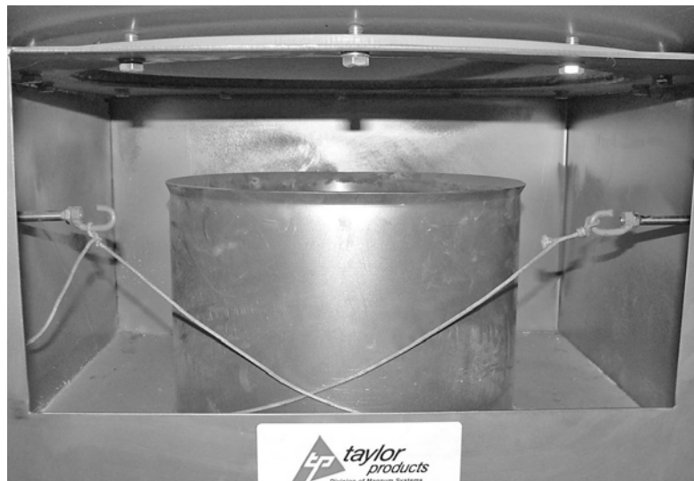
Figure 1-7. Drawstring and Drawstring Cylinder Hooks
