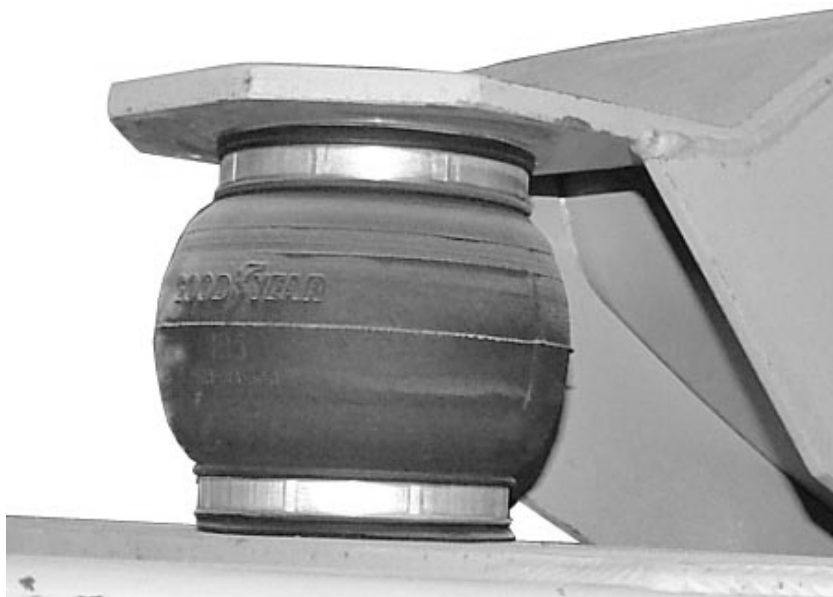
Figure 1-10. Optional Air Mount Isolator Pad (1 of 4 Shown)
