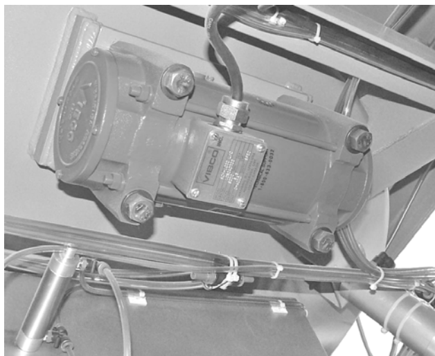
Figure 1-11. Vibrator Location (Electronic Vibrator Shown)
