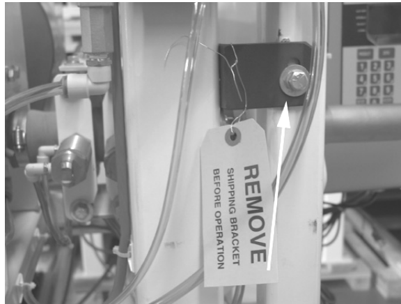
Figure 2-2. Shipping Brackets Connecting the Weigh Mast to the Main Frame
