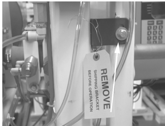
Figure 2-2. Shipping Brackets Connecting the Weigh Mast to the Main Frame
