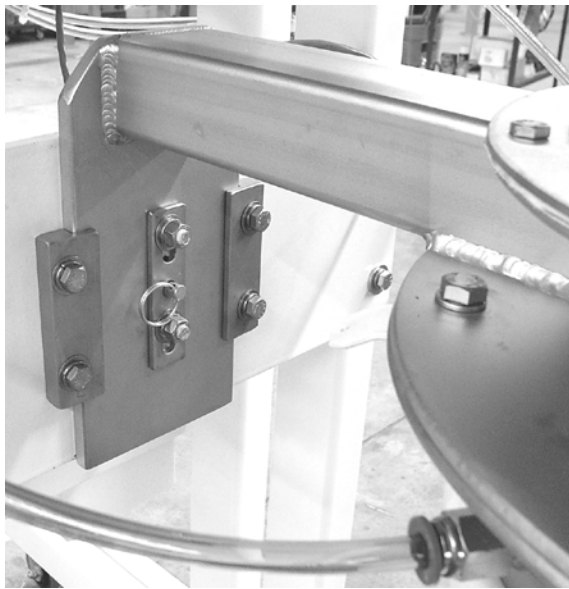
Figure 7-5. Open Mouth Bag Spout Mounting Bracket
