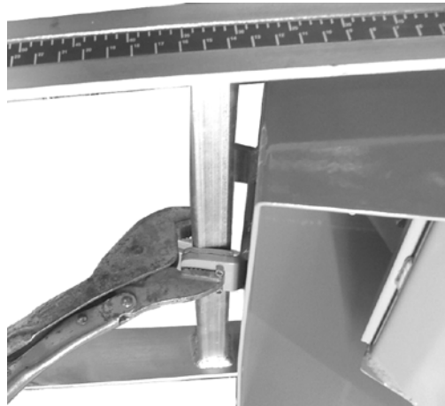
Figure 3-4. Clamping the Scale Beam Down
