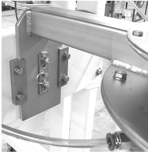
Figure 7-4. Open Mouth Bag Spout Mounting Bracket
